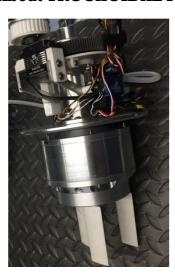
ADV TECH trochoidal propeller is a patented innovative rotor that permits a bio-mimetic "fish-like" motion of blades.
